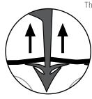
The lower anchor barb in a Roth Original Tacker E<sup>x</sup> clip is highly stable and equipped with a sharp cutting edge, while the anchor barb on top of this is exceptionally flexible. This special technology optimises the ease of installation.
