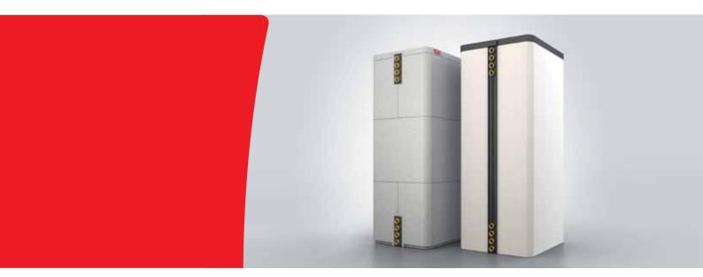
■ The corrosion-resistant Roth Thermotank Quadroline is made from a unique plastic composite material with aluminium diffusion protection and high-performance EPS insulation on the outside. It can withstand continuous pressure of 3 bar and a maximum operating temperature of 90 °C.
