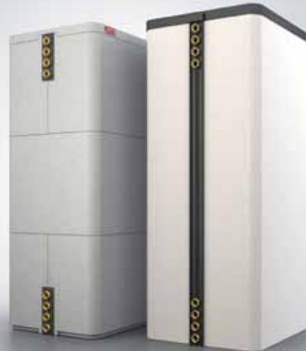
■ The corrosion-resistant Roth Thermotank Quadroline is made from a unique plastic composite material with aluminium diffusion protection and high-performance EPS insulation on the outside. It can withstand continuous pressure of 3 bar and a maximum operating temperature of 90 °C.
